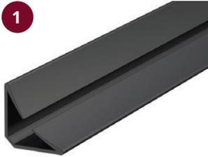
An acoustic and smoke perimeter seal which minimises the opening and closing resistance of the door leaf due to its unique, curved fins. Flexible elastomeric fin material springs back to original shape to provide ongoing performance and durability in service. Installed at the head and jambs of single and double leaf doors.
