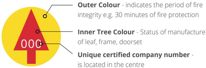
The plug to identify a Q-Mark accredited product will be located on the top of the door. The unique certified company number in the centre of the tree maintains traceability for which company was responsible for completing each part of the doorset manufacture, assembly and installation process. The unique number provides traceability to the Q-Mark scope certification.
